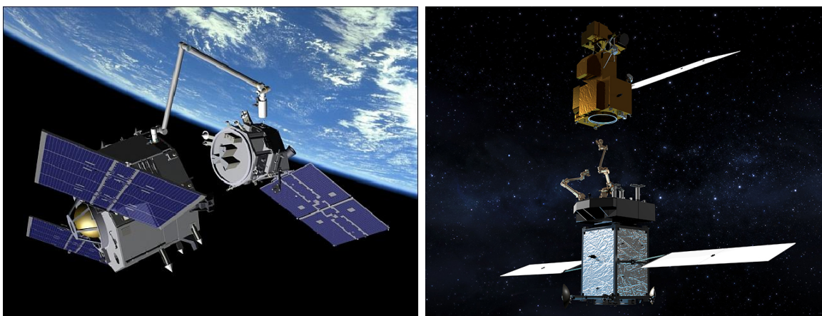
(a) Example grapple capture technologies proposed by MacDonald Dettwiler and Associates (b) NASA's Restore-L capture and servicing mission concept for Landsat.
